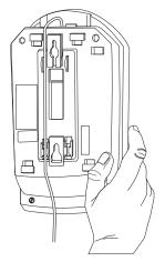
3. Plug the short telephone cord into the phone and the GTE Wall Plate jack. Place the Base Unit on the two posts of the wall plate and slide downward to secure.
